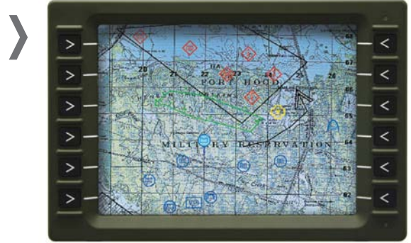
Figure 1 | The IEE 10.4-inch Thin Client Military Display uses an ARM processor and has dual-mode backlighting for night vision and sunlight readability.
